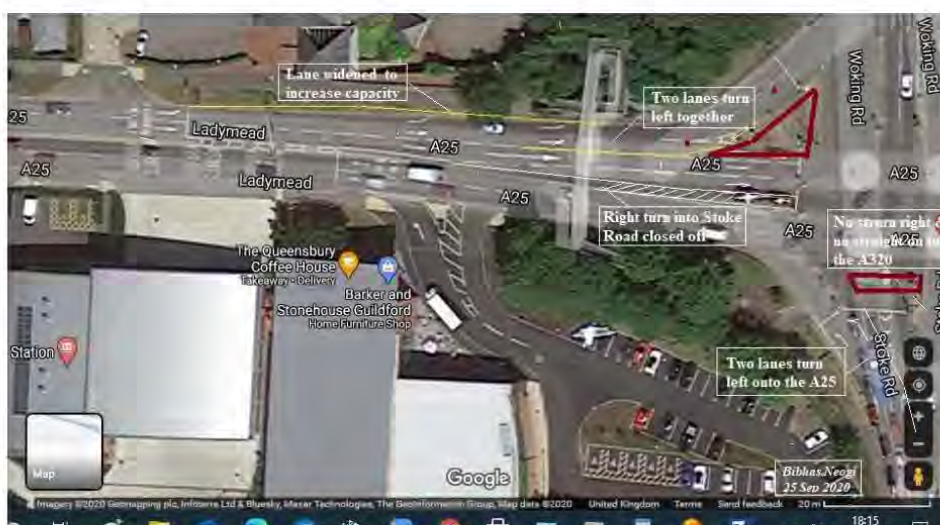
Altered Junction of the A25 & the A320 for better flow of traffic
