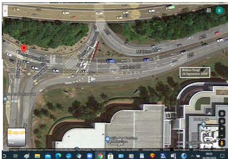
Alterations to lane exiting the roundabout onto Surrey Way.
