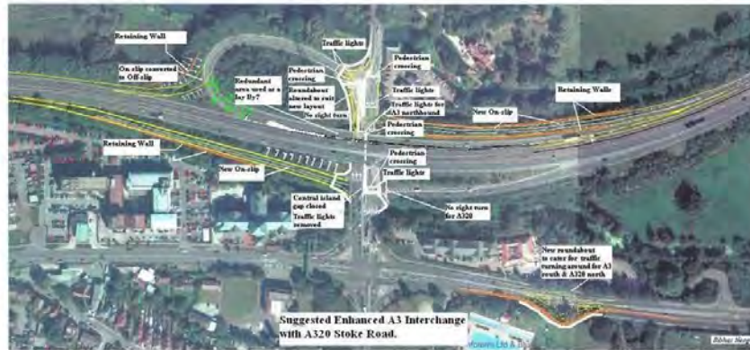
Modified Stoke Road Interchange and pedestrian routes
